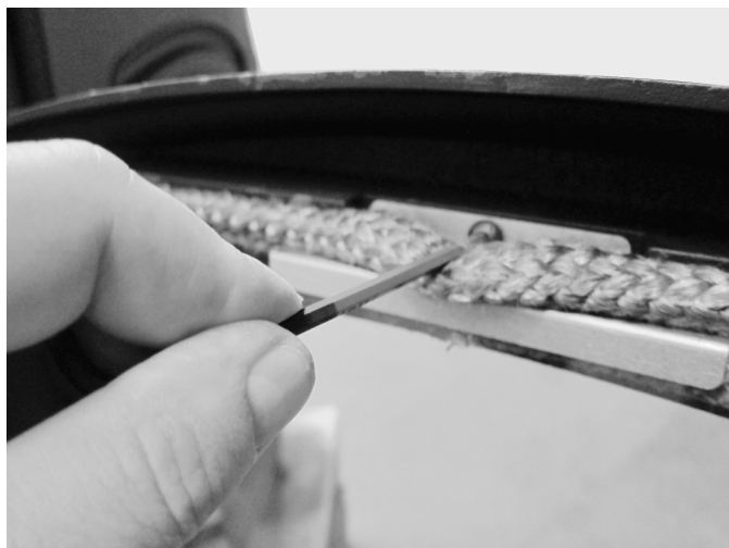
Figure 20. Loosen the glass clips.
