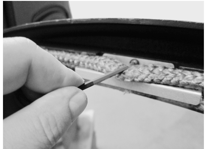
Figure 20. Loosen the glass clips.
