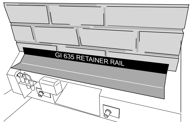
Figure 22 b. Brick panel lower retainer rail.
