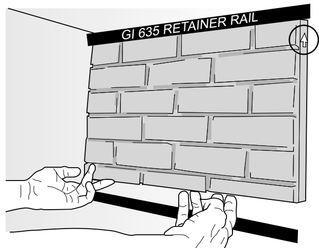
Figure 22 a. Install rear panel behind upper rail.
