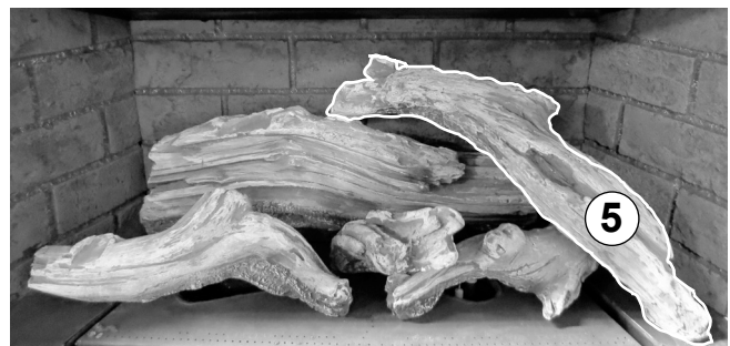
Figure 7.26. Engage the underside of Right Top Log #5 with Pin 5 indicated in fig. 7.25 as well as the matching seat on Log #1.
