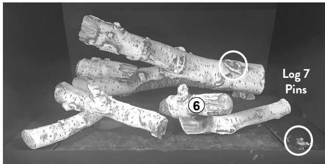
Figure 7.40. Engage matching notches in the underside of the Middle Cross Log #6 with the corresponding pins on Log #4 and the burner indicated in fig. 7.39.
