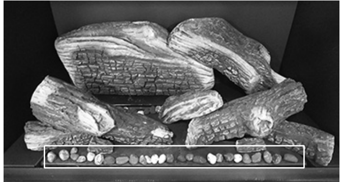
Figure 7.20 Position Burner Embers in row on burner. Be careful to avoid obstructing the pilot and burner carry-over ports shown in Fig. 7.21.
