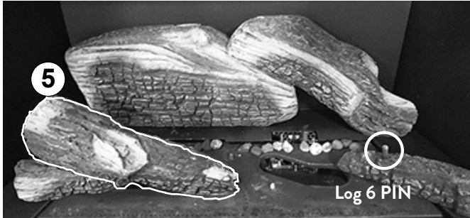
Figure 7.16. Engage holes in the underside of Left Cross Log #5 with the pin on Log #3 and the corresponding pin on the steel burner shown in fig. 7.15.
