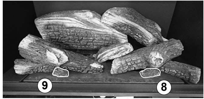
Figure 7.19. Position Right Small Log #8 and Left Small Log #9 in front of logs #5 & 6. Do not cover burner ports.
