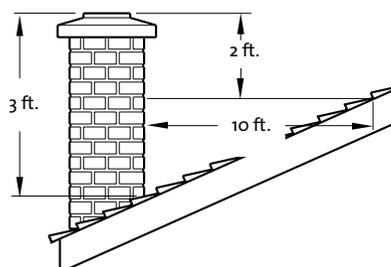
Figure 1. The 3' / 2' / 10' Chimney Rule.
