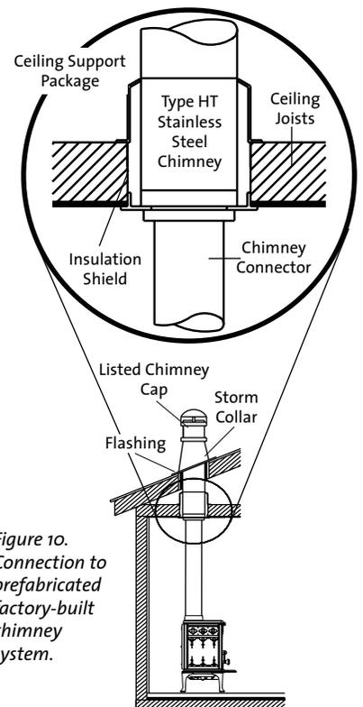
Figure 10. Connection to prefabricated factory-built chimney system.
