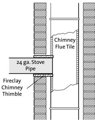
Figure 7. Chimney connection to a masonry chimney flue.
