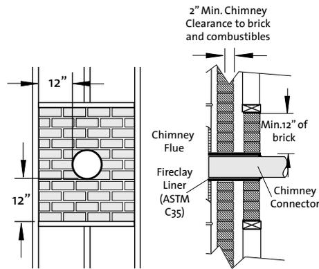
Figure 3. Bricked-in Fireclay Liner used as thimble
