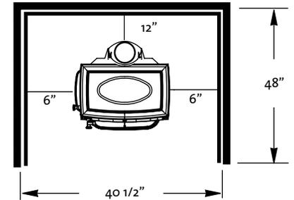
Figure 51. Alcove with protected wall clearances.
