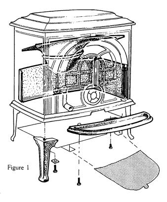
In order to prevent shipping damage, several parts of your stove have been removed and packed separately. These parts are:
